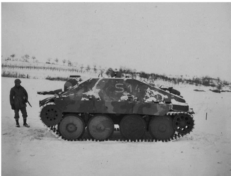
Figure 5: German JgPz38(t). Note the low silhouette and small size of this tank destroyer. Image credit: Pinterest
